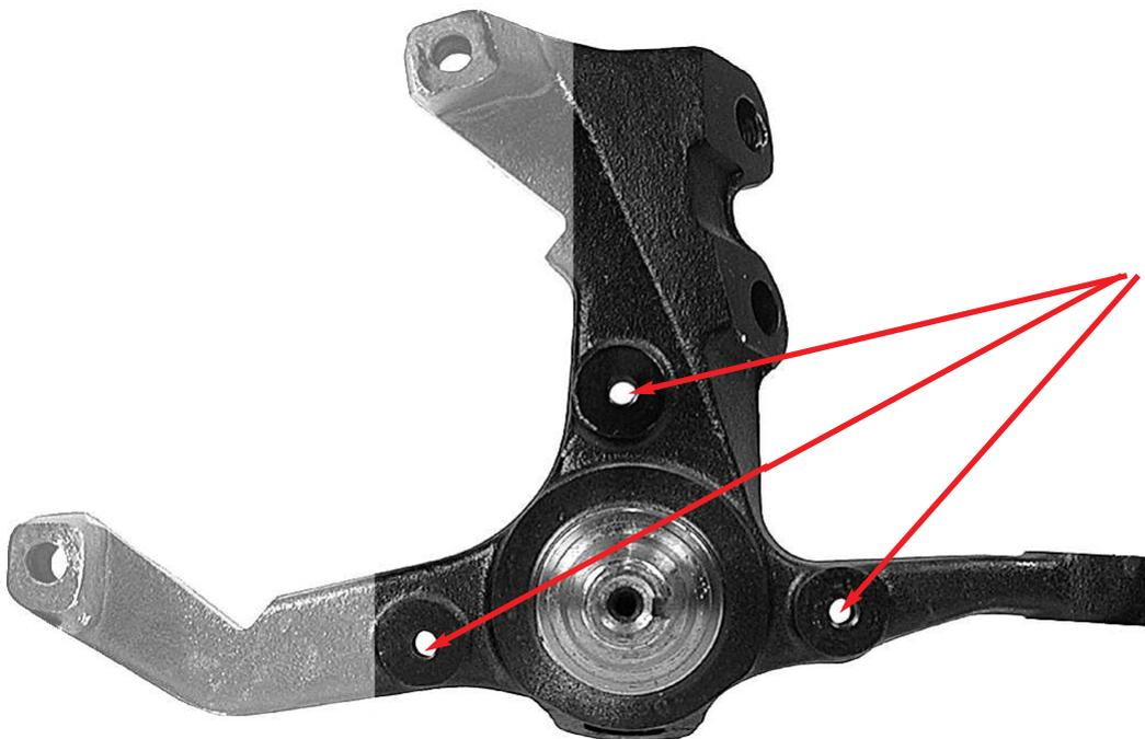
All 3 existing holes in spindle must be opened up to 7/16-20 thread with a .437 diameter counterbore .125 deep.
