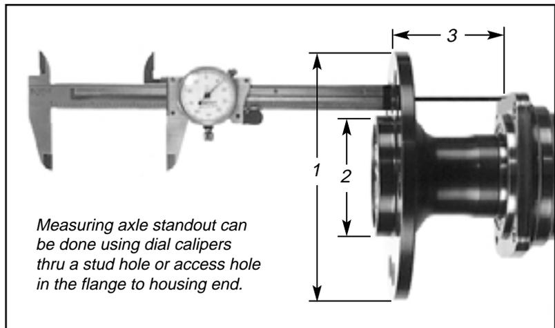
Measuring axle standout can be done using dial calipers thru a stud hole or access hole in the flange to housing end.
