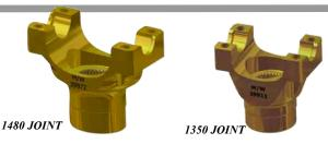
All MW aluminum yokes are CNC machined from 7075-T6 billet materials and have the MW Gold Coat process. These pinion yokes mate to the 39912 Gen II U-Bolt kits. Models are available for 1350 and 1480 series universals joints.
