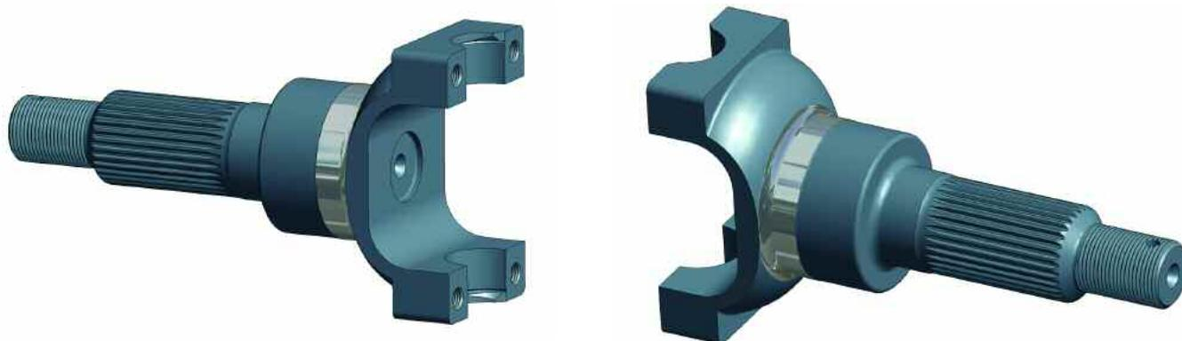
This is a fix for the early model Corvette rear hub shaft/yoke, that are prone failure. We have increased the spline size to a 31-tooth spline and the material is aircraft alloy steel thru-hardened for maximum strength. The threads are fine thread metric and comes with the nut and fine adjustment locking device. It does require boring and re-broaching you present hubs to 31-tooth spline, which we can do in house.
