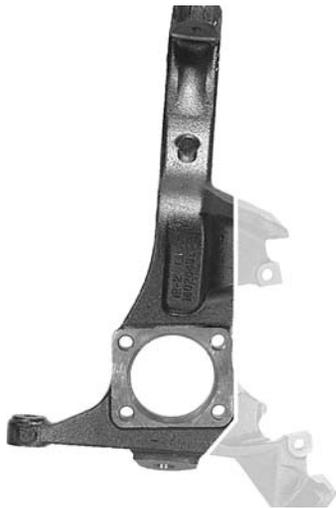
The spindle modifications required for the 75200/75250 brake kits are shown above. The faintly displayed material should be removed. Spindles can also be sent to Mark Williams Enterprises to have these modifications performed. If you have any questions call 303-665-6901, fax 303-665-7021 or e-mail to [info@mark-williams.com](mailto:info@mark-williams.com)
